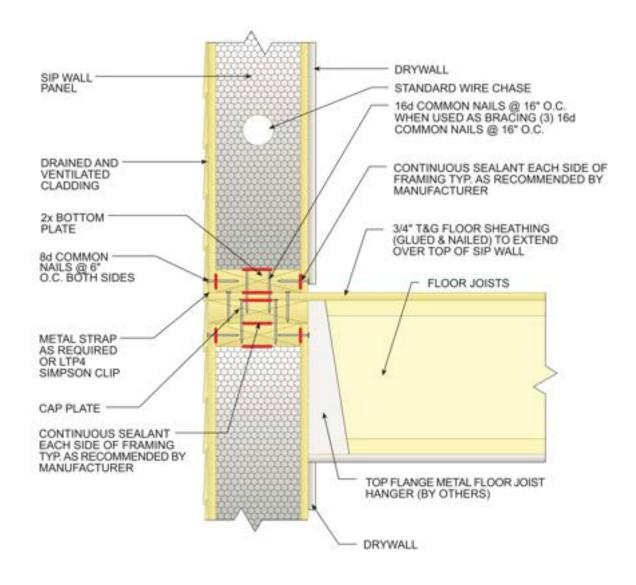
FOR SI: 1 inch = 25.4 mm. **Note:** Figures illustrate SIP-specific attachment requirements. Other connections shall be made in accordance with Tables R602.3(1) and (2) as appropriate.
