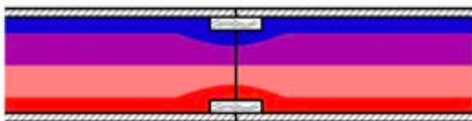
FIGURE 1.2: SIP WALL CROSS-SECTION WITH SURFACE SPLINE*
